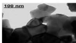
Figure 3: TEM Image of the Nanomaterial \text{Ni}_{0.2}\text{Cu}_{0.4}\text{Co}_{0.4}\text{Fe}_2\text{O}_4 annealed at 900^\circ\text{C}
